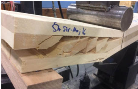
Photo 1: Flatwise Shear Failure - Major Axis 3-ply
