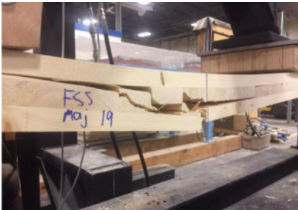
Photo 2: Flexural Bending Failure - Major Axis 3-ply
